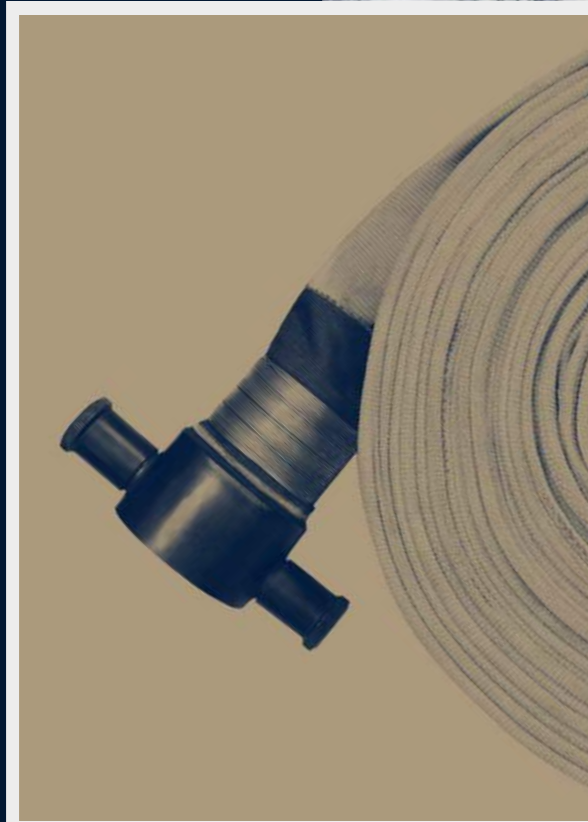
ROLLED LEATHER HOSE WITH SCREW COUPLINGS
